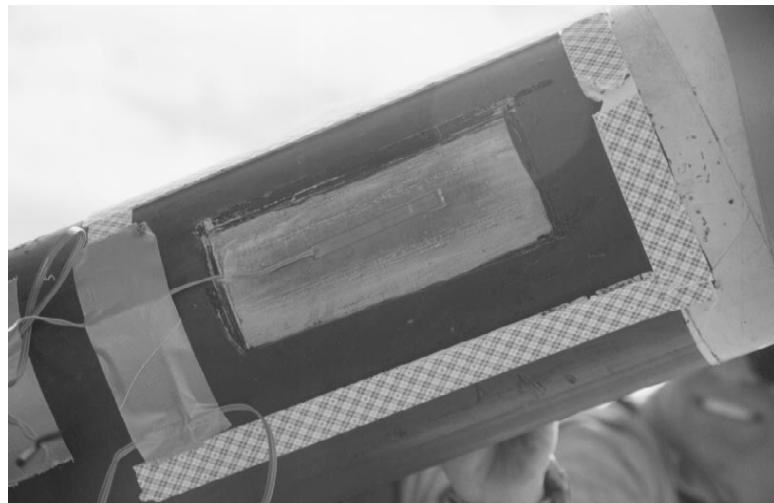
Figure 3.14: Strain Gage Applied to Grout Surface
