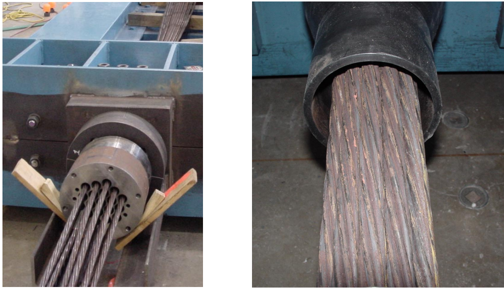
Figure 7.1: Installation of Strand During Construction of Stay Cable Specimen
