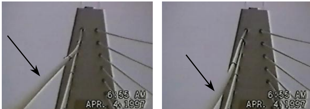
Figure 3.6: Peaks of Motion from a Video of Vibration of Cable A24S on the Fred Hartman Bridge
