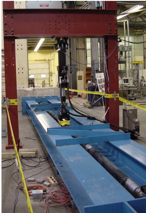
Figure 7.2: Stay Cable Bending Fatigue Test
